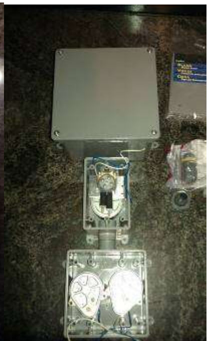
Pumps hardwired in (not remote)
