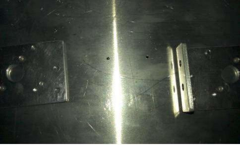
All drilled. Brackets are mounted. Long screws through the pump faceplate that you removed earlier from the FRONT of the housing cover:
