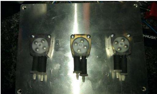
Mount the corresponding pump on to the bracket with the short screws. The shafts are 'keyed' and you remember which faceplate went to which pump...
