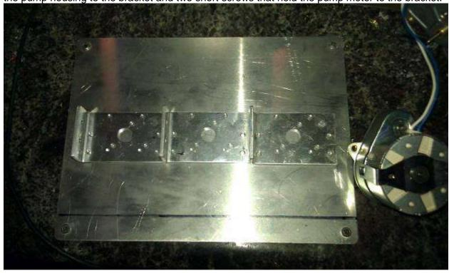
Use your marker to mark screw holes for the LONG screws and the large center hole (for pump shaft) only. The short screws are internal to the box.
