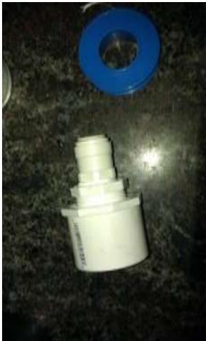
Wrap your other Watts connector threads and install it into the ½" threaded
