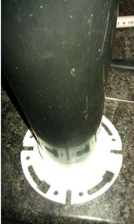
Put it in the sink, fill it with water and 'leak test' your fittings, especially the bottom.
