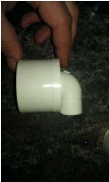
Now glue your  $\frac{3}{4}$ " PVC tube through the reducer, into the  $\frac{3}{4}$ " slip elbow you just glued into the
