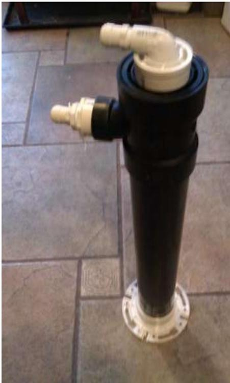
Install your hose, cut to length and attach to your pump. The top hose goes to the pump. Bottom hose just goes back to the reservoir.
