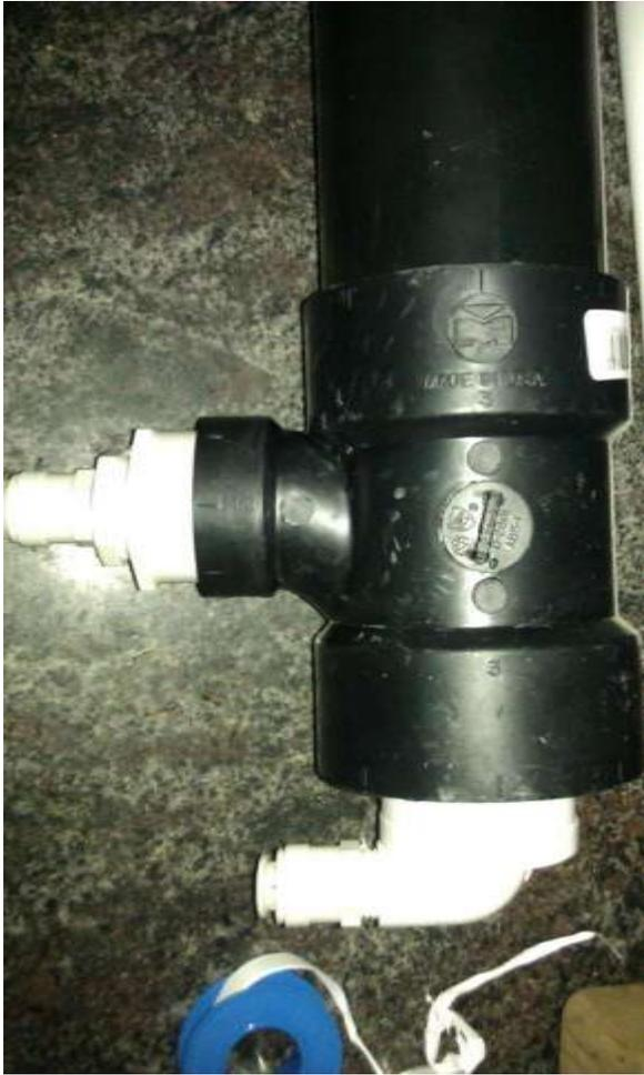
Install/glue the 3" 'Tom - Kap' drain fitting on the bottom of your 3" PVC. When you are sourcing parts, look for one that fits 'snug' in the tube you will be using. Mine was slightly loose and leaked initially. Worst case, glue your rubber gasket between the pipe end the tom kap lip. Trim gasket as needed.
