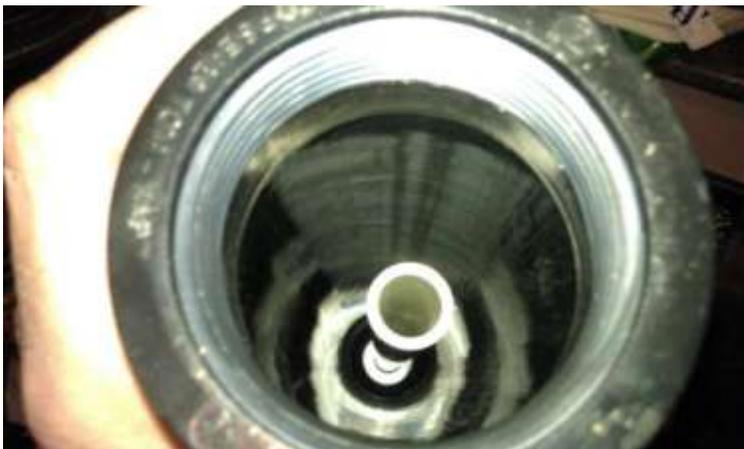
Start shoving your scrubbies down the pipe. Alternating them so you don't create 'path' for the water, either up the center or along the pipe side. I put in a few layers of plastic ones, then did all the stainless
