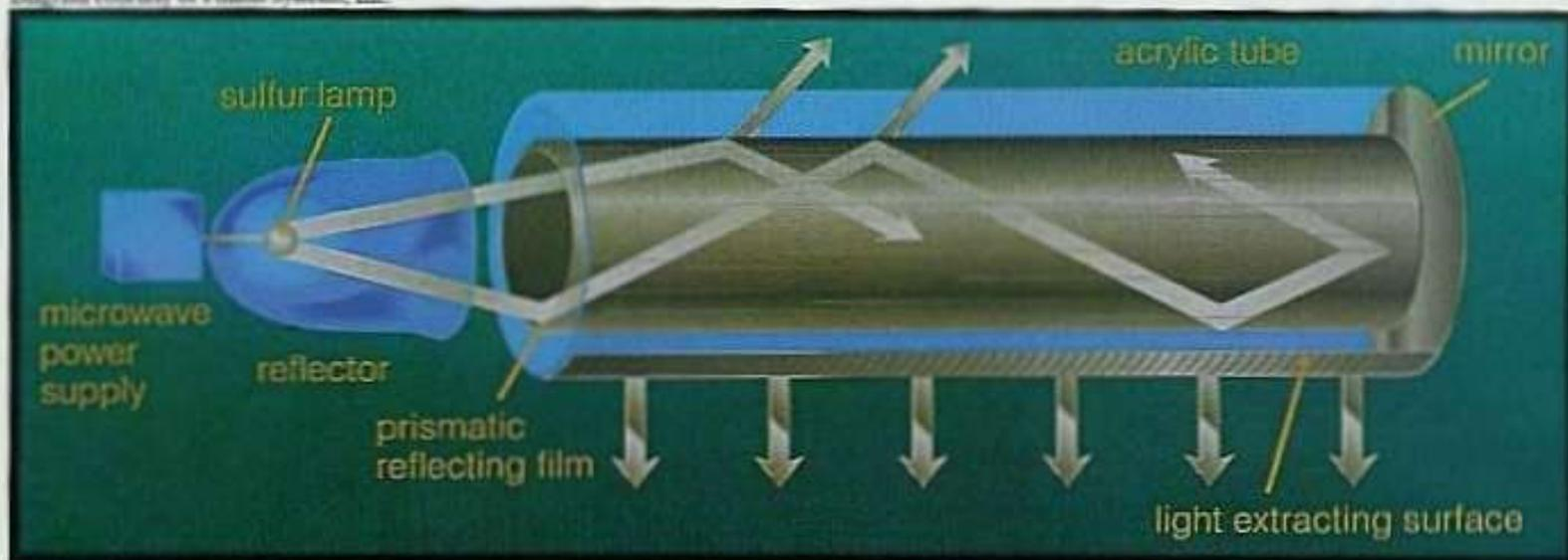
Each sulfur bulb contains an inert gas and a small amount of sulfur. When the sulfur is bombarded with microwave energy, it forms a plasma that emits light very much like sunlight. The lamp can be used in a variety of different configurations. On the opening page of this article it is shown with a reflector. In the diagram above it is pictured with a light pipe. In either configuration, it can be filtered, tinted, dimmed and reflected to meet the unique lighting requirements of any facility.
