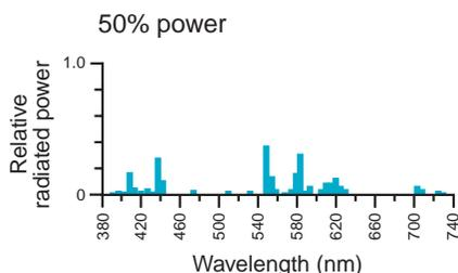
SPD curves for a 400-watt, coated high-pressure sodium lamp
